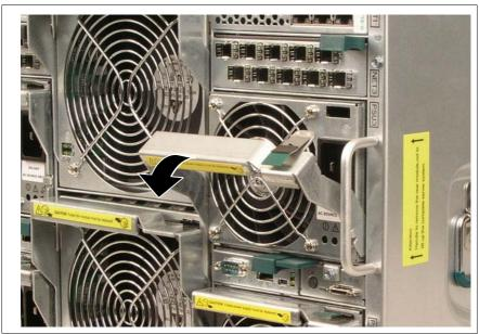
Figure 78: Removing the power supply unit
